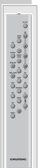
ON/OFF Switches the hi-fi system to standby mode and from standby mode to the last signal source
